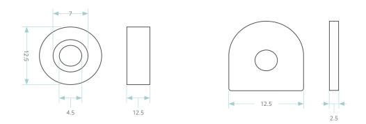
\*Magnets are attached to the shutter panel. Striking plates are attached to the frame.
